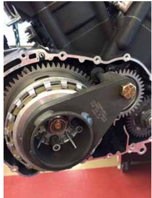
Figure 5-9. CLUTCH LOCKING TOOL
