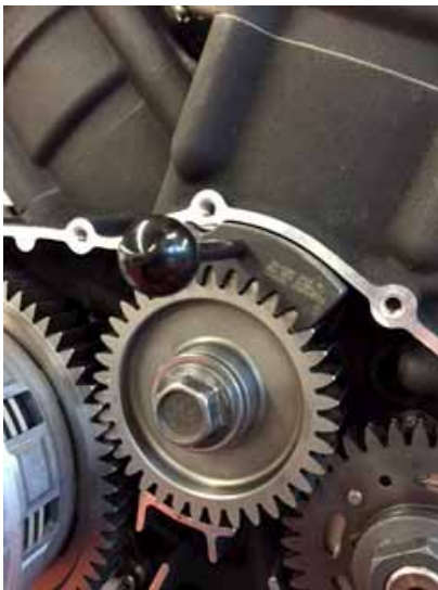
Figure 4-37 CRANKSHAFT LOCK HD-51281 installed
