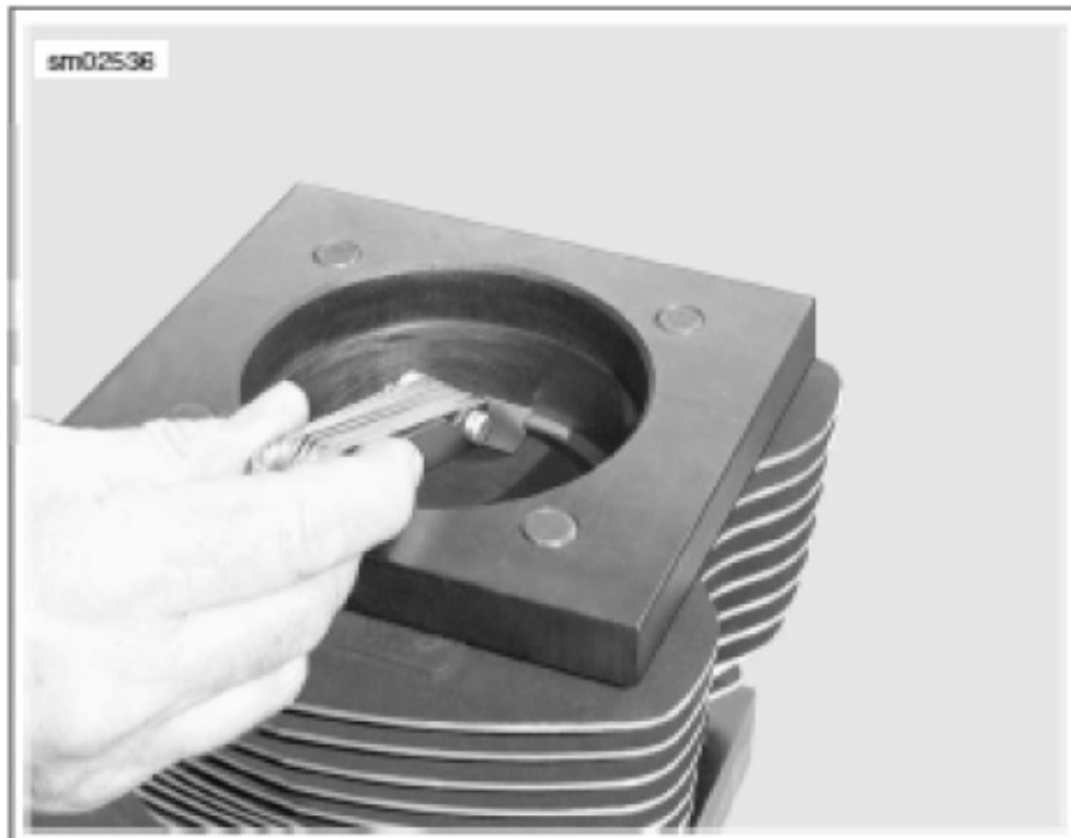
Figure 3-62. Measuring Ring Gap
